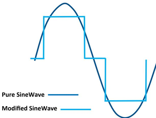
Inverters are available with either a square/stepped/quasi or Pure Sinewave Output. The former is an approximation of an AC Sinewave. Suitable only for running simple loads like a mono-filament lamp, they will cause overheating, possible damage and poor performance of sophisticated loads like microwaves, power tools, audio visual equipment etc.
